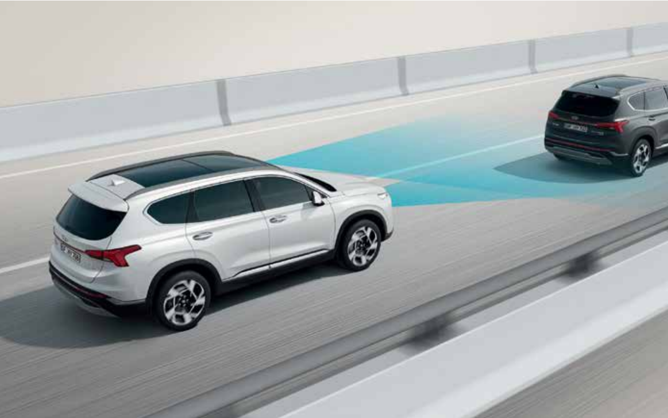
Highway Driving Assist (HDA) Keeps you centred in your lane and traveling at a safe distance behind the car ahead when Smart Cruise Control or Lane Following Assist is active.
