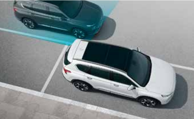
Blind-Spot Collision-Avoidance Assist (BCA) Using radar sensors in the lower rear bumper and a front camera, the system warns you of traffic in the blind spot area. Should you set the turn indicator in such a situation, it will sound an acoustic alert and brake to prevent collision. Safe Exit Assist (SEA) This clever feature prevents accidents by detecting vehicles approaching from behind and temporarily locking the rear child lock doors, so that passengers can only exit the car when it is safe to do so.
