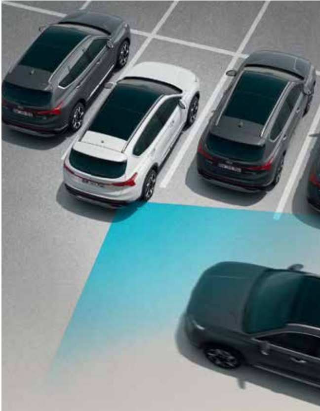
Rear Cross-Traffic Collision-Avoidance Assist (RCCA) When reversing out of areas with low visibility, the system not only warns the driver if vehicles approach from the side – it also applies the brakes automatically.
