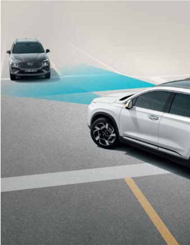
Forward Collision-Avoidance Assist (FCA, junction turning) The FCA system warns you and automatically brakes when it detects sudden braking by the car ahead or detects pedestrians or cyclists in your path. The same applies to collision risks with oncoming vehicles while turning left at an intersection.
